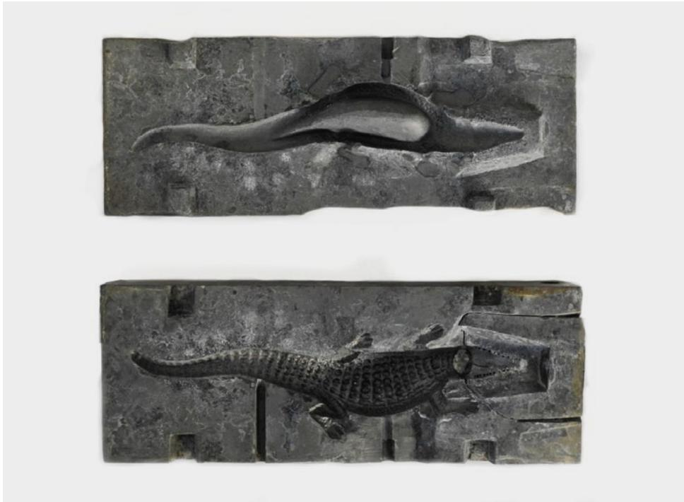
These moulds were probably used to create animal figures as part of a manufacturing workshop. Die casting is a metal casting process that is characterized by forcing molten metal under high pressure into a mould cavity. The mould cavity is created using two hardened tool steel dies (in this instance the shape of a gorilla and crocodile) which have been machined into shape and work similarly to an injection mould during the process.
